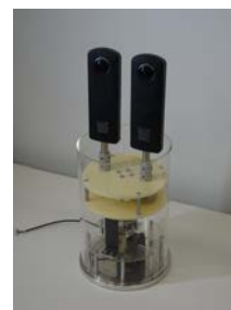
Figure 2: TwinCam head (fixed-azimuth rotation mechanism).
